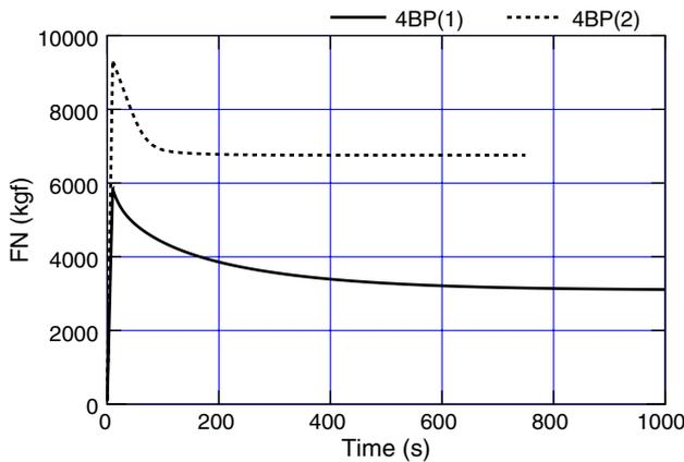
Fig. 12 Rudder force in the 4BP series
