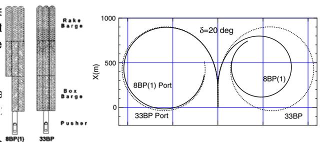
Fig. 14 Turning trajectories of 8BP(1) and 33BP
