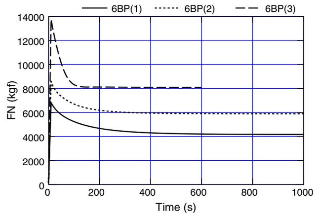
Fig. 13 Rudder force in the 6BP series
