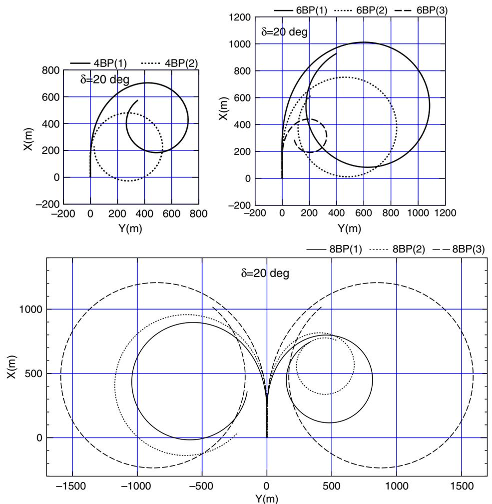
Fig. 11 Tactical diameter and advance distance( $\delta=20$ )
