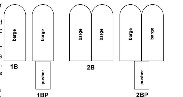
Fig. 15 Pusher-barge systems with and without pusher
