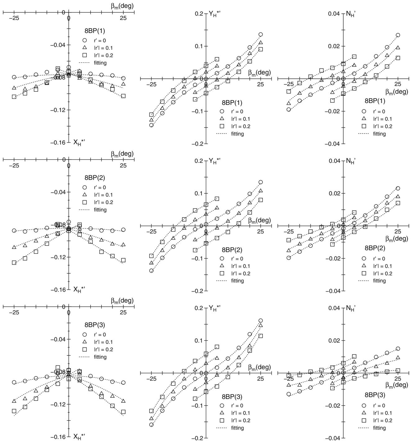
Fig. 8 Measured force and moment coefficients for 8BP(1), 8BP(2), and 8BP(3)
