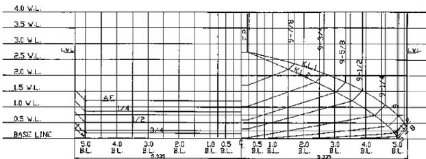
Fig. 3 Body plan of the rake-barge
