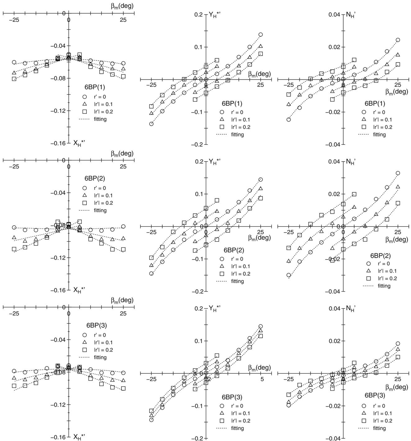
Fig. 7 Measured force and moment coefficients for 6BP(1), 6BP(2), and 6BP(3)
